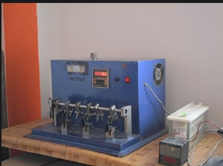
UPPER MATERIAL TEST RIG
